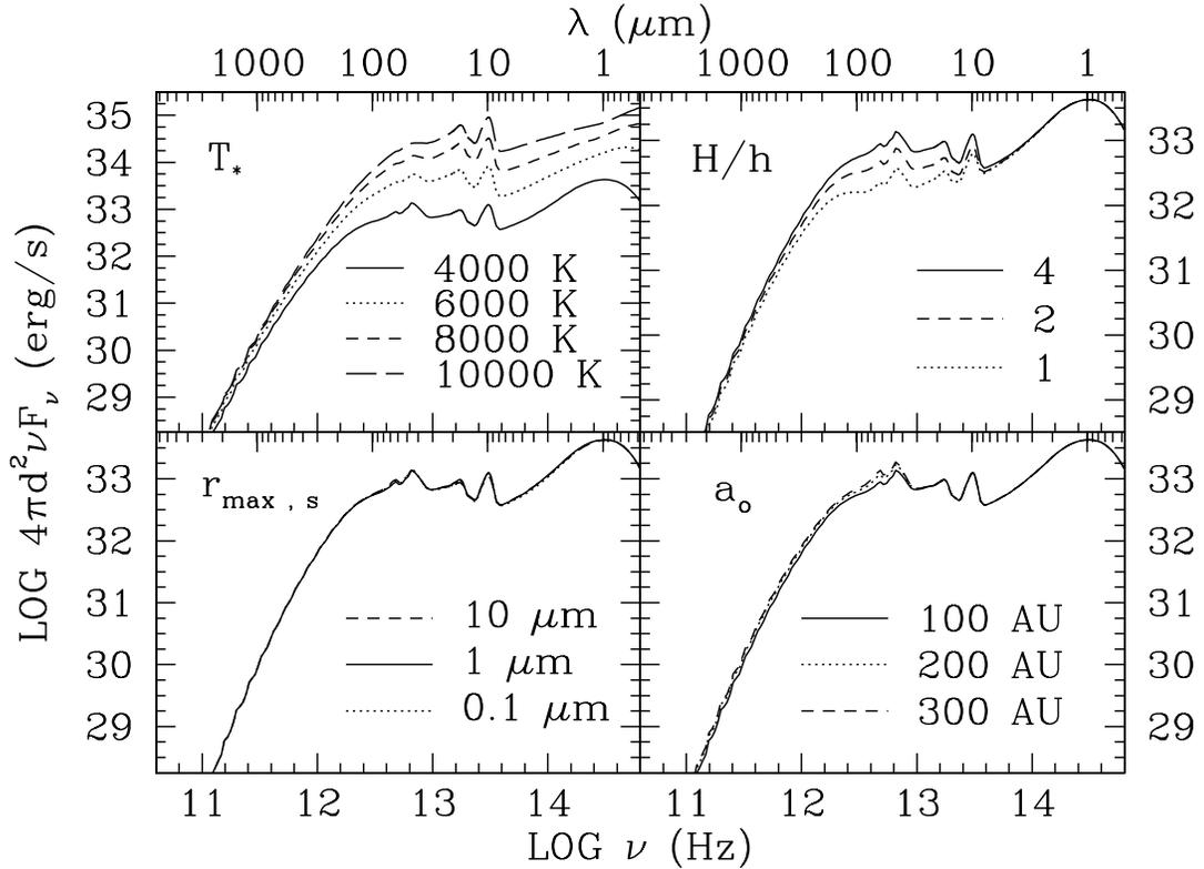
FIG. 8.—Dependence of SED on input parameters  $T_*$ ,  $H/h$ ,  $r_{\max,s}$ , and  $a_o$ . In each panel, the indicated parameter takes on several values, while all other parameters are fixed at their standard model values.
