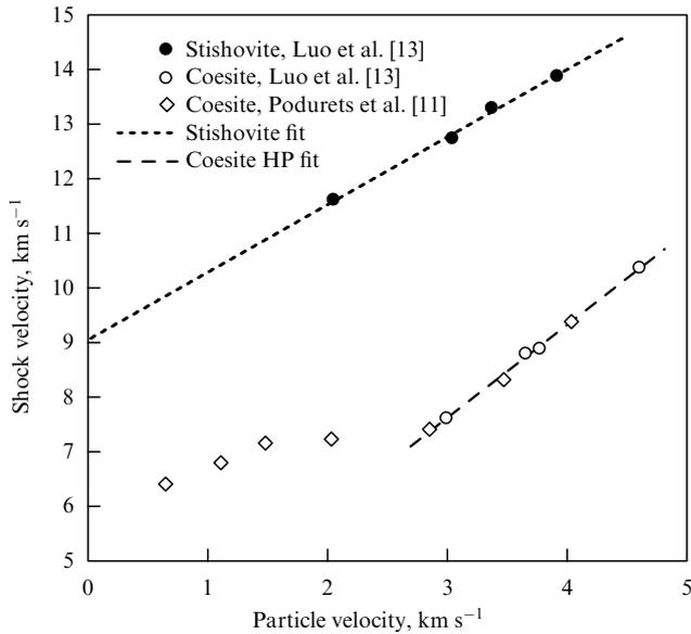
**Figure 1.**  $U_s - u_p$  relationships for stishovite and coesite [11, 13]. Stishovite:  $U_s$  (km s<sup>-1</sup>) = 9.08 + 1.23  $u_p$ ,  $\rho_0 = (4.31 \pm 0.04)$  g cm<sup>-3</sup>. Coesite in high-pressure regime (HP):  $U_s$  (km s<sup>-1</sup>) = 2.52 + 1.70  $u_p$ ,  $\rho_0 = (2.92 \pm 0.03)$  g cm<sup>-3</sup>.
