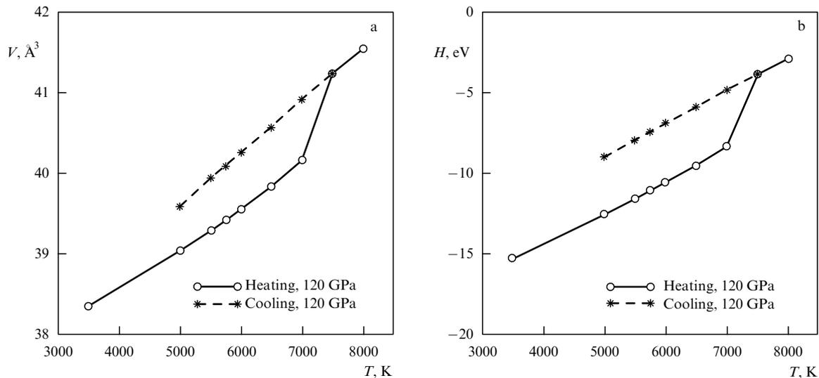
**Figure 5.** Single-phase simulation of stishovite melting at 120 GPa with molecular dynamics [14]. (a) The unit cell (2 SiO<sub>2</sub> formulae) volume, and (b) the corresponding enthalpy during the heating–cooling process.
