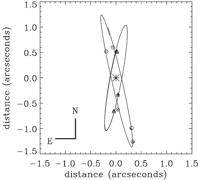
FIG. 2.—Projected orbits of the two satellites of 2003 EL61. Observations of both satellites and their measurement errors are shown. The predicted locations of the distant satellite (circles) and the close satellite (triangles) at the times of observation are also shown. For an assumed circular orbit of the inner satellite, the best fit gives an orbital period of  $34.7 \pm 0.1$  days and a relative inclination between the two satellites of  $39^\circ \pm 6^\circ$ .
