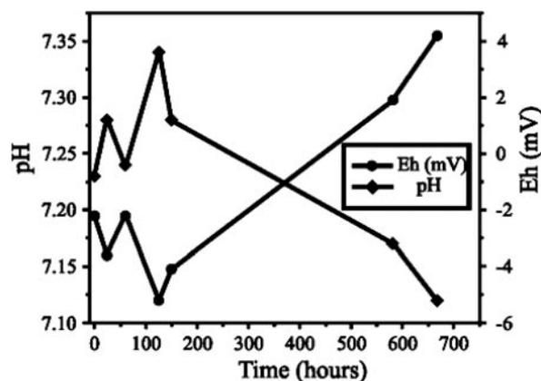
**Fig. 1.** Time-course analysis of pH and Eh showing minimal variation of both pH (7.10–7.35) and Eh (–4 to +4 mV) throughout the experiment. Note that the system becomes slightly oxidizing after 400 h, when magnetite becomes the predominant phase.
