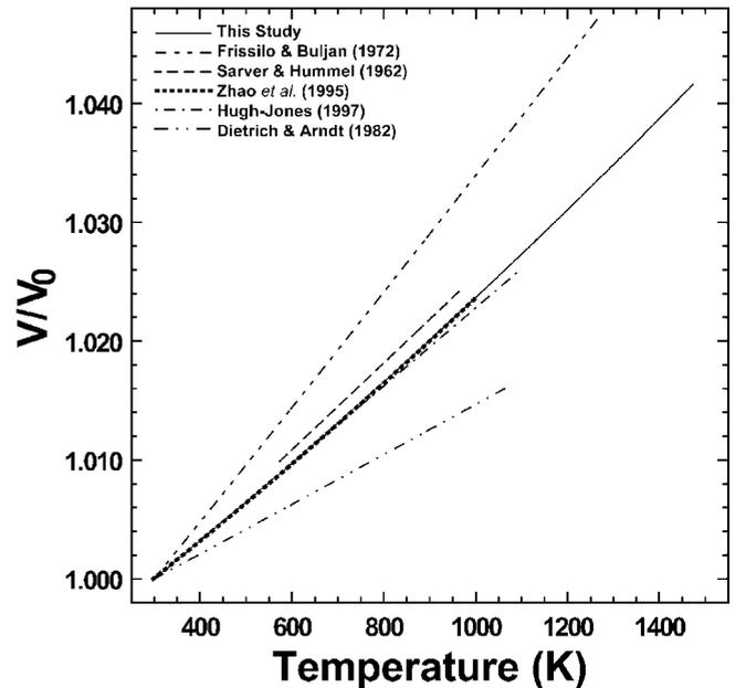
Fig. 3. Normalized volume thermal expansion curves of orthoenstatite from previous measurements. The curves for this study and Zhao *et al.* (1995) are calculated using a linear temperature dependence for  $\alpha(T)$  (Table 1).
