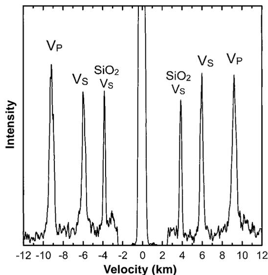
FIGURE 3. Brillouin spectrum of  $\gamma\text{-Mg}_2\text{SiO}_4$  collected at 873 K.
