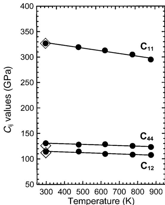
**FIGURE 5.** Single crystal elastic moduli of  $\gamma$ -Mg<sub>2</sub>SiO<sub>4</sub> as a function of temperature. Circles = this study; diamonds = Weidner et al. (1984).
