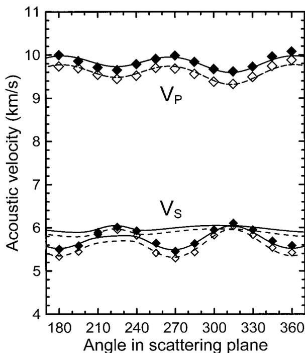
FIGURE 4. Measured acoustic velocities as a function of angle in the scattering plane at 298 K (solid symbols) and 773 K (open symbols). The lines show acoustic velocities calculated from the best fit single-crystal elastic moduli (solid line for 298 K and dashed line for 773 K).
