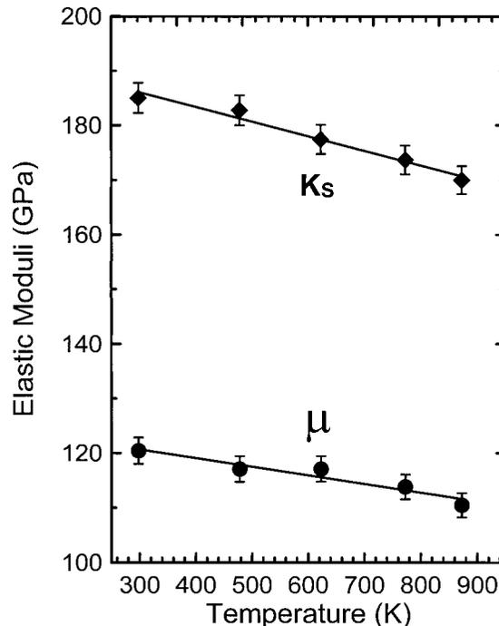
**FIGURE 6.** Aggregate elastic moduli of  $\gamma$ -Mg<sub>2</sub>SiO<sub>4</sub> as a function of temperature.
