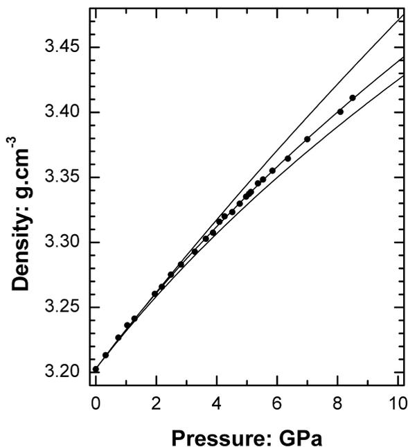
**FIGURE 1.** The variation with pressure of the density of MgSiO<sub>3</sub> orthopyroxene. Points are the  $P$ - $V$  data collected by Angel and Hugh-Jones (1994). The lines represent various equations of state, from top:  $K_{T0} = 106$  GPa and  $K'_0 = 4$ ,  $K_{T0} = 102.3$  GPa and  $K'_0 = 9.2$ ,  $K_{T0} = 106$  GPa and  $K'_0 = 10.7$ .
