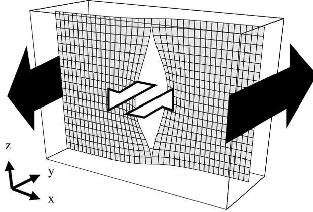
Figure 1: Geometry of the antiplane shear problem.
