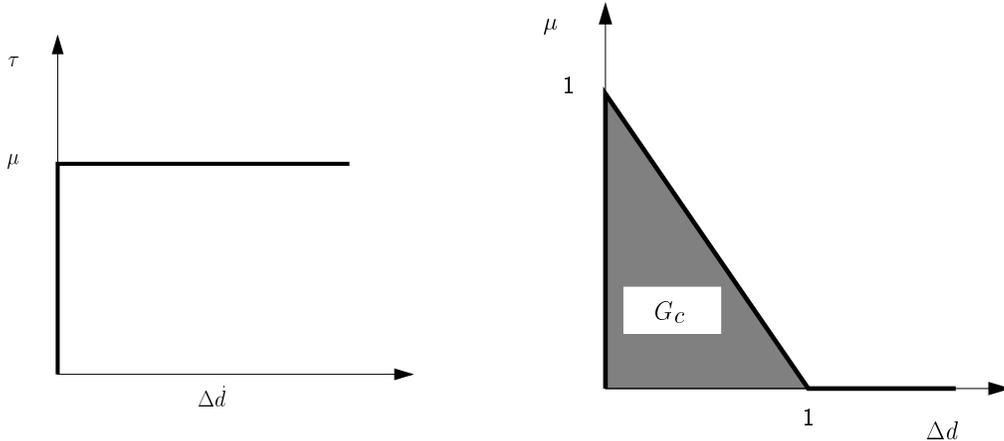
Figure 2: (a) Friction graph relating fault stress  $\tau$  to slip rate  $\Delta\dot{d}$ .  $\mu$  is the current friction coefficient (also called here fault strength). (b) Linear slip weakening friction law prescribing the evolution of  $\mu$  with ongoing slip  $\Delta d$ . The fracture energy  $G_c$  is the area of the shaded surface. All quantities are dimensionless.
