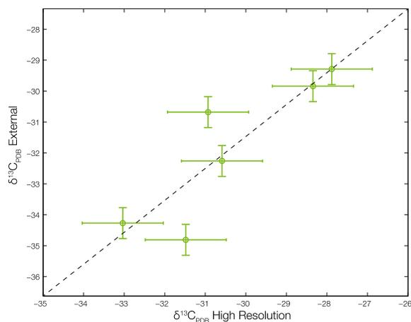
Fig. 5. Plot of bulk molecular  $\delta^{13}\text{C}$  value of representative natural samples calculated from our measurements of methyl and ethyl fragment ions (horizontal axis) versus those measured independently by GC-combustion—IRMS (vertical error bars assume an estimated  $\pm 0.5\%$  for these external measurements).
