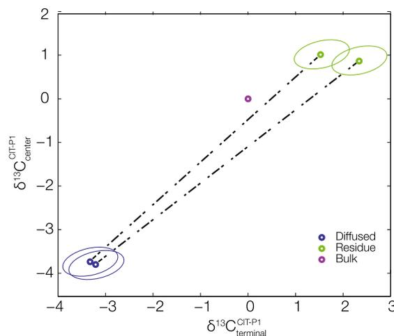
Fig. 7. Results of two diffusion experiments of propane through a needle valve. No site-specific preference was expected or measured, and the measured offset between the diffused gas and residue is within error of the expected value.
