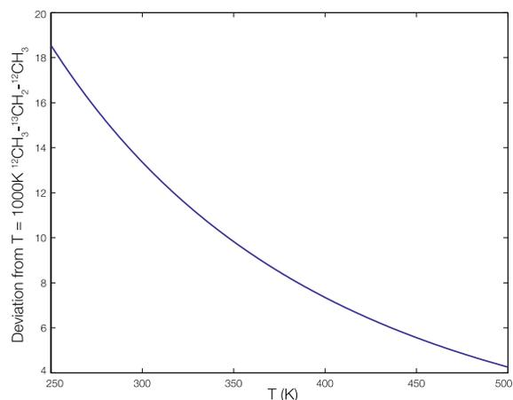
Fig. 6. Predicted relationship between the enrichment in  $^{13}\text{C}$  in the center position of propane relative to the terminal positions (vertical axis, units are 1000.Ineq for Reaction (7)) and temperature (horizontal axis, in kelvin). Equilibrium isotope effects tend to concentrate  $^{13}\text{C}$  in the central position, by  $\sim 5\text{--}15\%$  over geologically relevant temperatures, with a temperature sensitivity that may be suitable for geothermometry.
