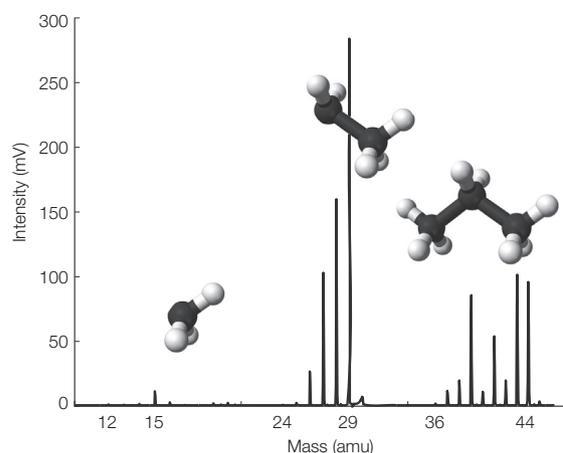
Fig. 1. Mass spectrum of propane from the MAT 253 Ultra, collected using a faraday cup registered through a 10<sup>8</sup> Ω amplifier. The structures of major fragment and molecular ions are illustrated with ball and stick figures.
