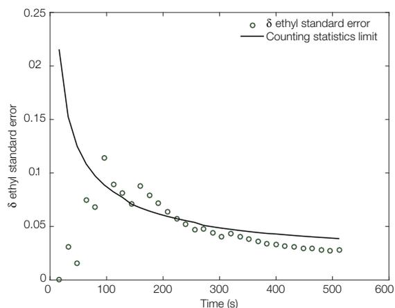
Fig. 3. Shows the relationship between counting time for the 2-carbon ethyl measurement, and the counting statistics limit. Average cumulative measurement time is for entire length of figure. Therefore the counting statistics limit is typically reached.
