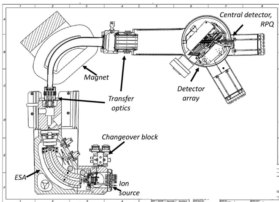
**Fig. 1.** Schematic illustration of the major components of the source, analyzer and detector array of the Thermo 253-Ultra. The changeover block is a set of pneumatic valves through which one of the 5 possible streams of analyte gas or carrier gas flows to the ion source. Other major labeled components include the Nier type electron impact ion source, the electrostatic analyzer (ESA), magnet and detector array. Not to scale.
