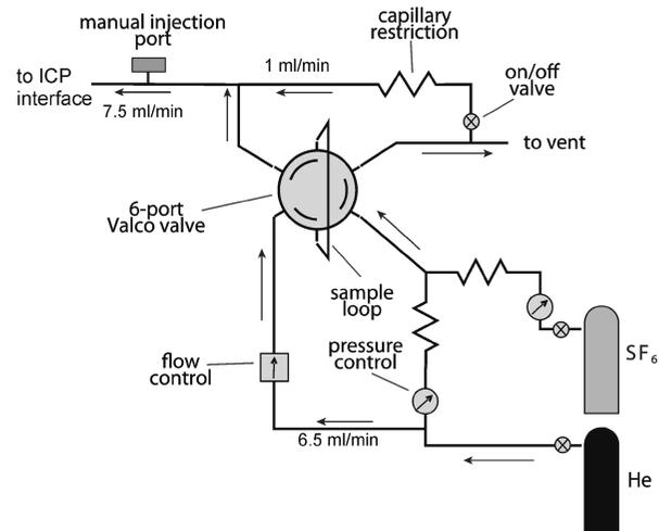
**Figure 2.** Schematic layout of the apparatus used to introduce a continuous flow or discrete peaks of SF<sub>6</sub> reference gas at variable concentrations. Reference gas is 2% SF<sub>6</sub> in He and is further diluted to ~250 ppm SF<sub>6</sub> in He (~50 ppm S). This gas is used for instrument tuning, testing, and calibration of analyte isotope ratios.
