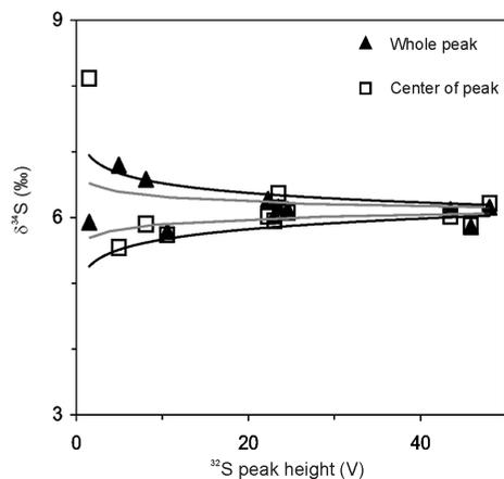
**Figure 6.** Values of  $\delta^{34}\text{S}$  for hexylthiophene as a function of peak height. Triangles are the integration of the whole peak, whereas squares are integration of the center of the peak. The gray ( $1\sigma$ ) and black ( $2\sigma$ ) lines represent limiting precision based on ion-counting statistics.
