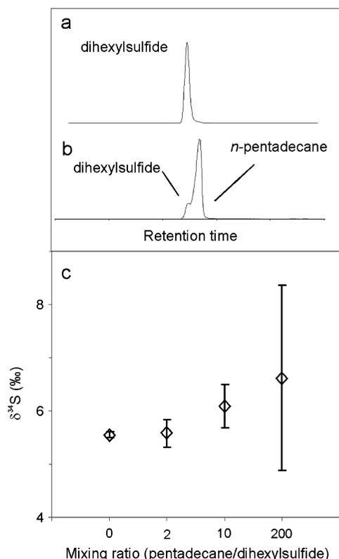
**Figure 7.** Effect of a hydrocarbon coeluting with the organosulfur analyte: (a)  $^{32}\text{S}$  trace measured by GC/ICPMS; (b) TIC (total ion current) trace measured by GC/MS; (c)  $\delta^{34}\text{S}$  values ( $1\sigma$ ,  $n = 3$ ) of dihexylsulfide measured by GC/ICPMS.  $\delta^{34}\text{S}$  values were calibrated against an internal standard (hexylthiophene) that elutes at a different time.
