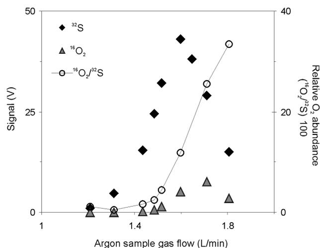
**Figure 4.** Effect of Ar sample gas flow rate on sensitivity and  $\text{O}_2^+$  formation for  $\text{SF}_6$  (50 ppm S in He). Diamonds are  $^{32}\text{S}$  intensity in volts, triangles are  $^{16}\text{O}_2$ , and circles represent the  $^{16}\text{O}_2/^{32}\text{S}$  ratio (right axis).
